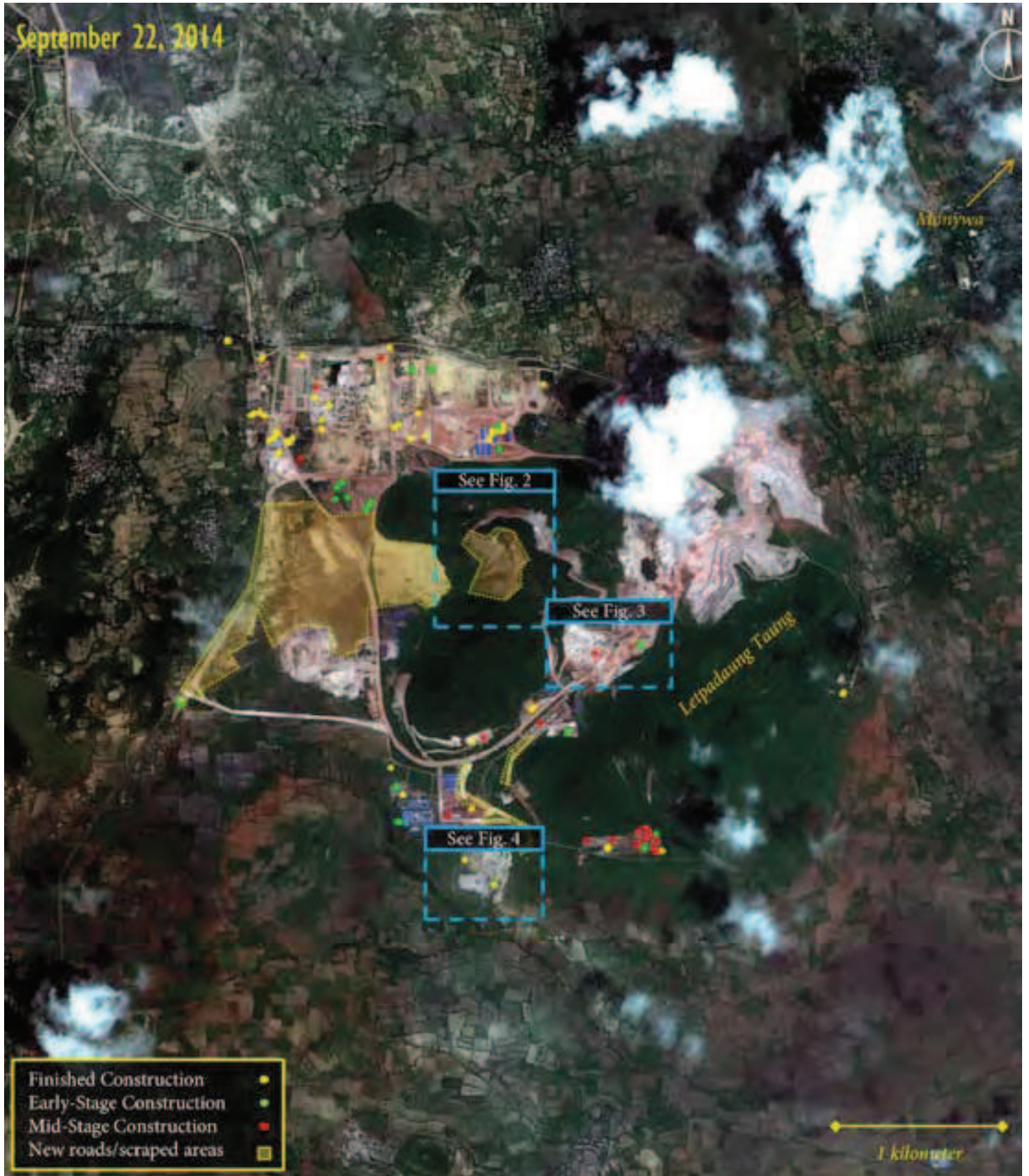
fig 1: Approximately 18 square kilometers of the mining area near Monywa, Myanmar, were analyzed for major changes in infrastructure and other activity between May 14 and September 22, 2014. Of the 87 structures recorded, 50 were considered completed (roofs finished), 28 in early-stage construction and 9 still under construction. DigitalGlobe September 22, 2014, 22.081°,95.088°
