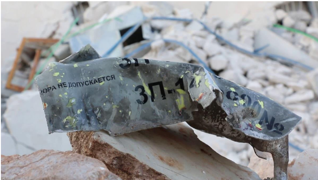
Remnant of Russian Kalibr cruise missile. Still taken from video © Darat Izza Media Office.
