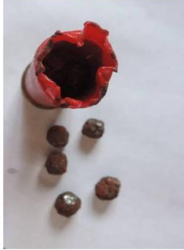
Top: Hunting cartridges modified by removing the original pellets (lead shots) and replacing them with bigger artisanal shots (seized from anti-Balaka in Carnot). Bottom Hunting cartridges modified by inserting machine gun cartridge 7.62x54R shown on the left (seized from anti-Balaka in Bouar)
