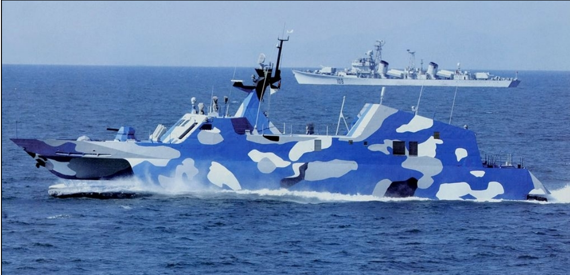
Figure 10. Houbei (Type 022) Class Fast Attack Craft With an older Luda-class destroyer behind
