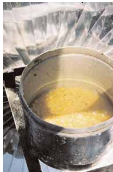
Parabolic solar cooker being used in Beldangi I camp.
