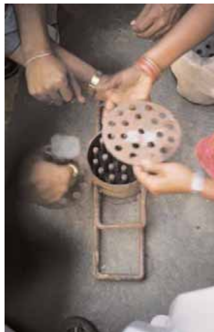
Trainee demonstrating the use of the single-briquette press for the honeycomb briquette.
