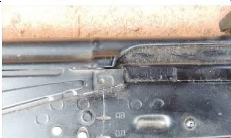
Fire selector indication of Soviet origin
