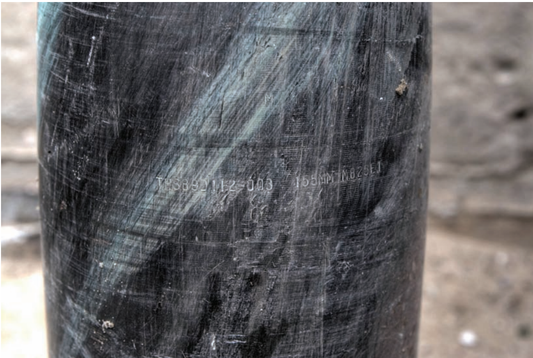
A 155mm white phosphorus artillery shell streaked with the telltale light green paint used on these shells. This shell was manufactured by Thiokol Aerospace in the United States in April 1989. The M825E1 stamping is the US Army designation for a white phosphorus shell containing 12.74 pounds of phosphorus, which burns at up to 1500 degrees Fahrenheit (816 degrees Celsius). © 2009 Marc Garlasco/Human Rights Watch
