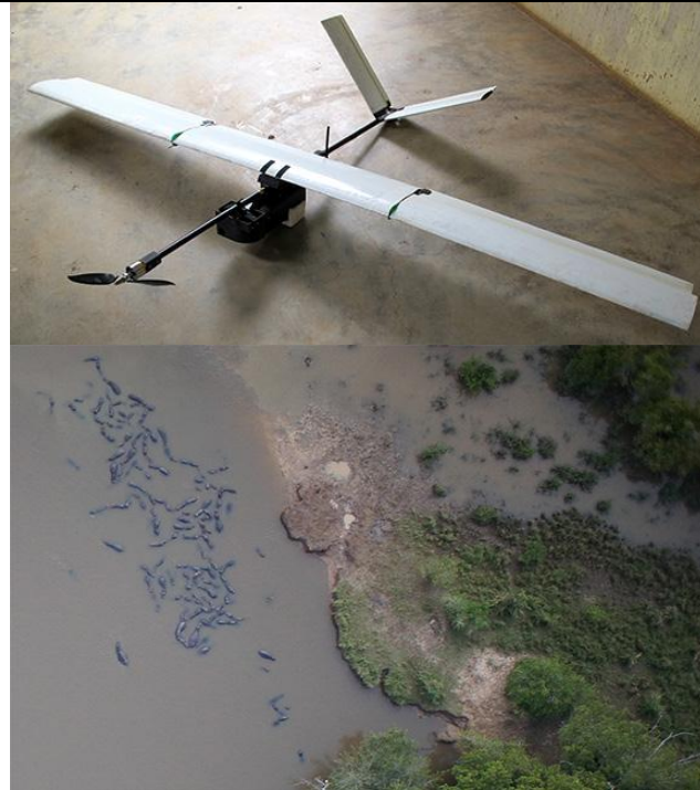
The drone has a wingspan of 2.5 meters and weighs 6 kg, with the camera. The image above (bottom) shows a photo taken by the drone, of hippos in a river in Garamba park.
