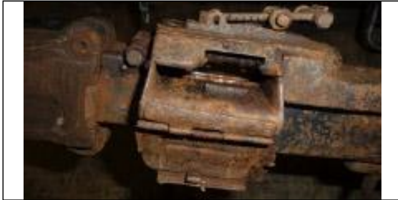
Belt receiver of a PKM 7.62x54mm calibre general-purpose machine gun. Photo taken in Mwenga, South Kivu, 5 September 2014.
