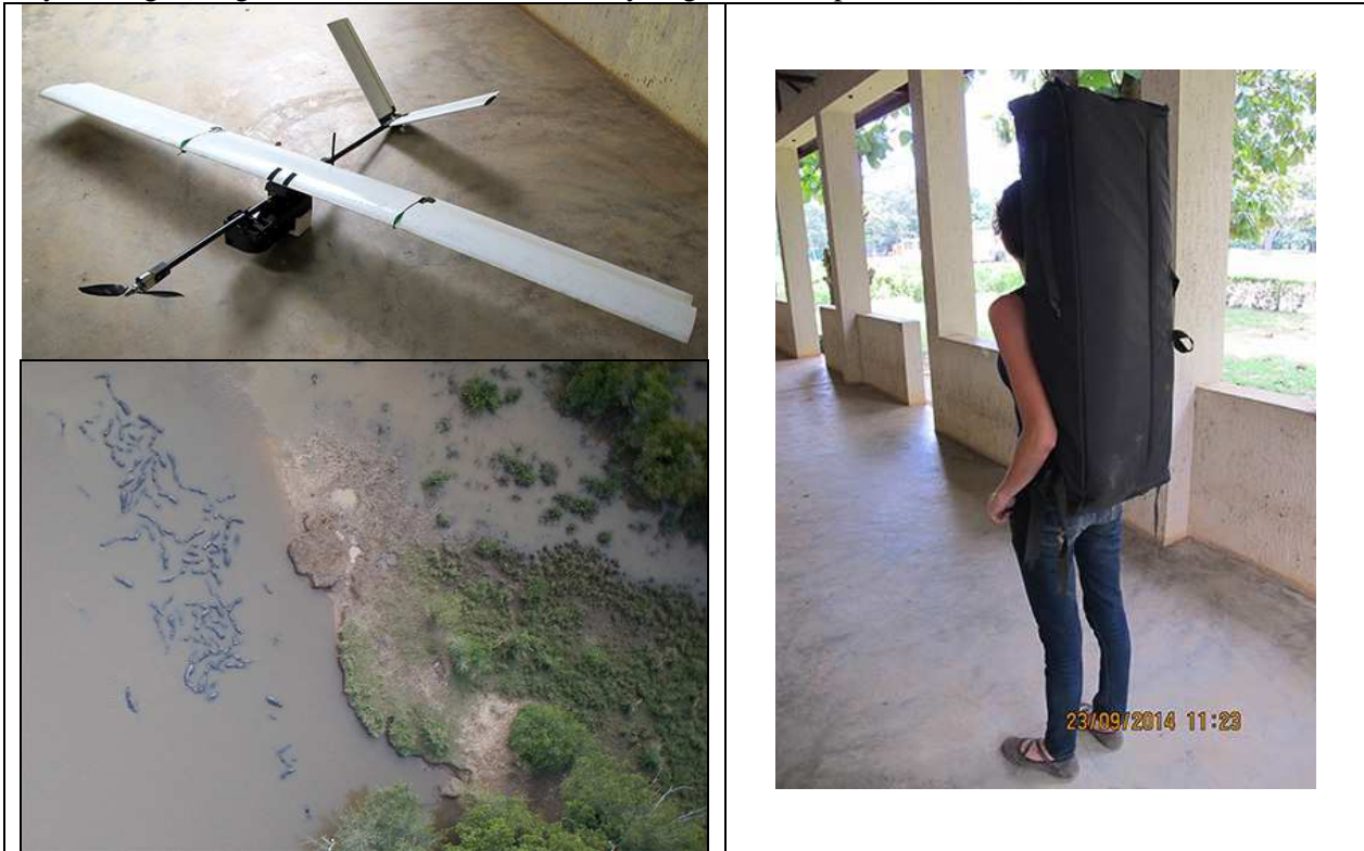
The drone has a wingspan of 2.5 meters and weighs 6 kg, with the camera. The image above (bottom) shows a photo taken by the drone of hippos in a river in Garamba park.
