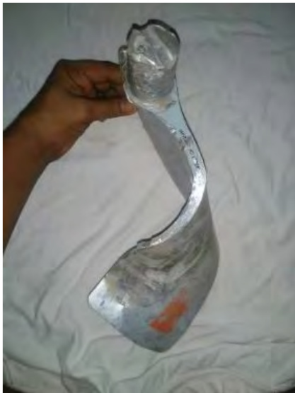
Figure 49.B.4 Post-explosion guidance fin from a Paveway laser guidance system
