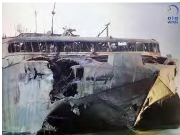
Figure 13.4 Exit point of ASM Port Midships
