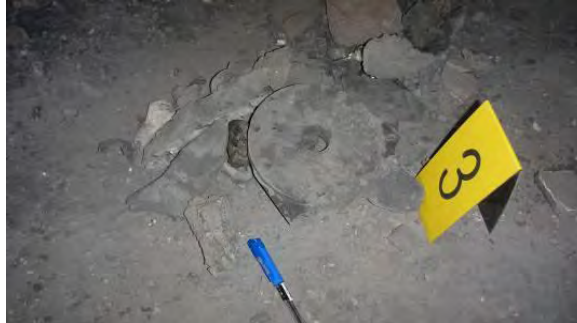
Figure 49.D.9 GBU-12 PAVEWAY II guidance unit wing fragment in situ 301
