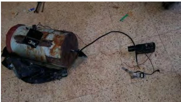
Figure 43.5 EFP Radio-Controlled IED (RCIED), Al Mukalla (16 May 2016)
