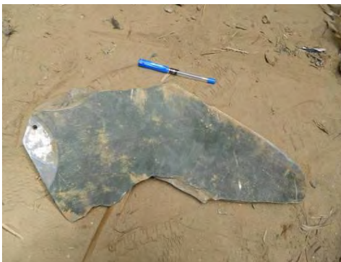
Figure 49.A.2 Rear fin from PAVEWAY terminal guidance unit 216
