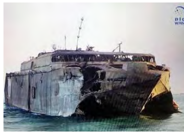
Figure 13.5 Fire damage to aluminium superstructure on Port Bow
