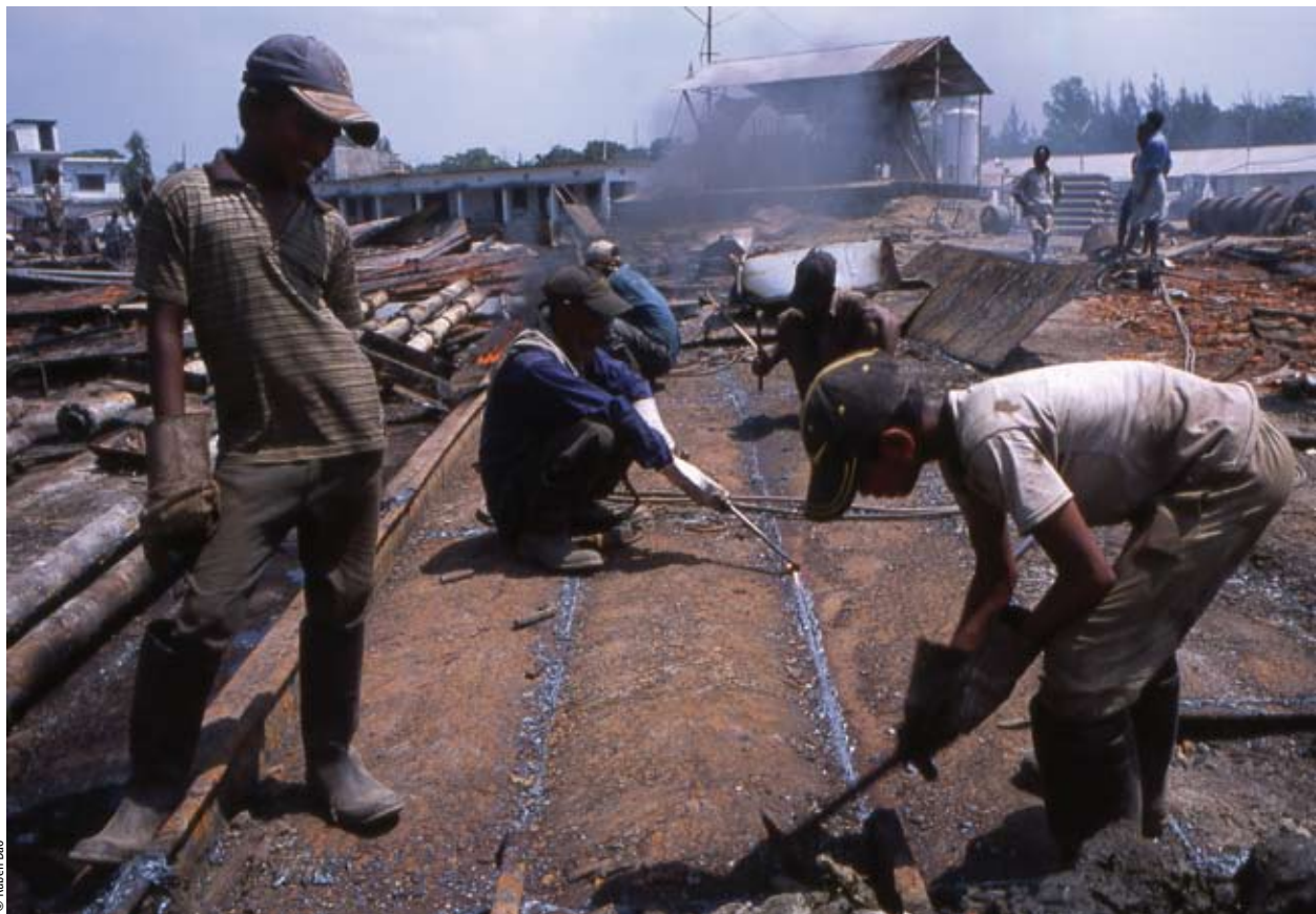
A child working as cutter helper cleans an iron plate to be cut from its rust.
