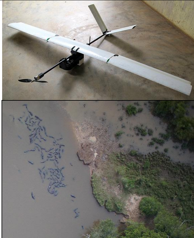
The drone has a wingspan of 2.5 meters and weighs 6 kg, with the camera. The image above (bottom) shows a photo taken by the drone of hippos in a river in Garamba park.
