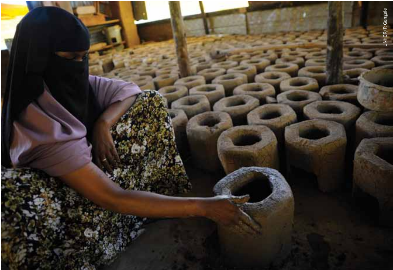
Making fuel-efficient stoves in Hagadera camp, Dadaab, Kenya. Fuel-efficient stoves require investment by assistance organisations but reduce the impact on the local environment.
