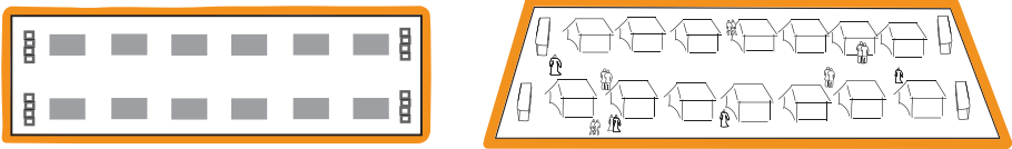
Image 17: Short double lines with communal latrine blocks at the end
