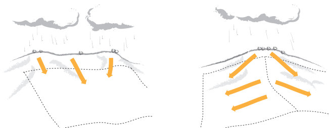
Image 36: The first step is to identify where the water will go
