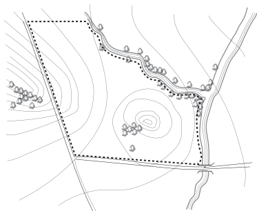
Image 33: Most sites come in irregular shapes, it is important to first mark the perimeter
