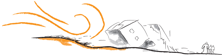
Image 8: Houses built on exposed piece of land can be vulnerable to extreme wind
