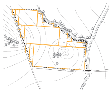
Image 34: Dividing the site into rectangles and squares help ease the calculation
