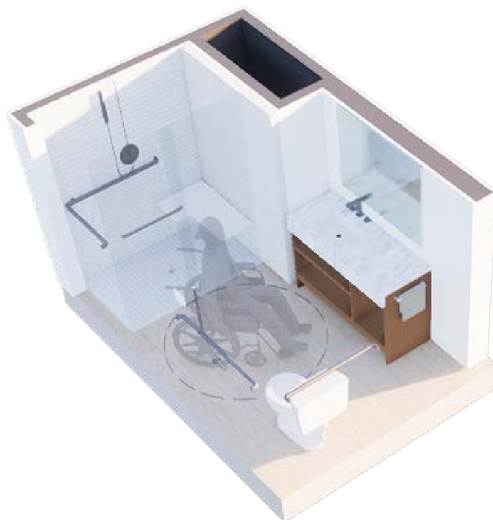
Figure 54: Accessible hotel bathroom 3D layout
