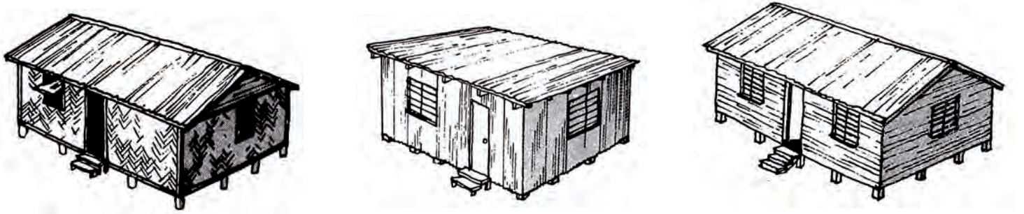
Wall types of transitional timber-framed housing (from left to right): with woven mats, CI sheets and timber boards (©Intertext)
