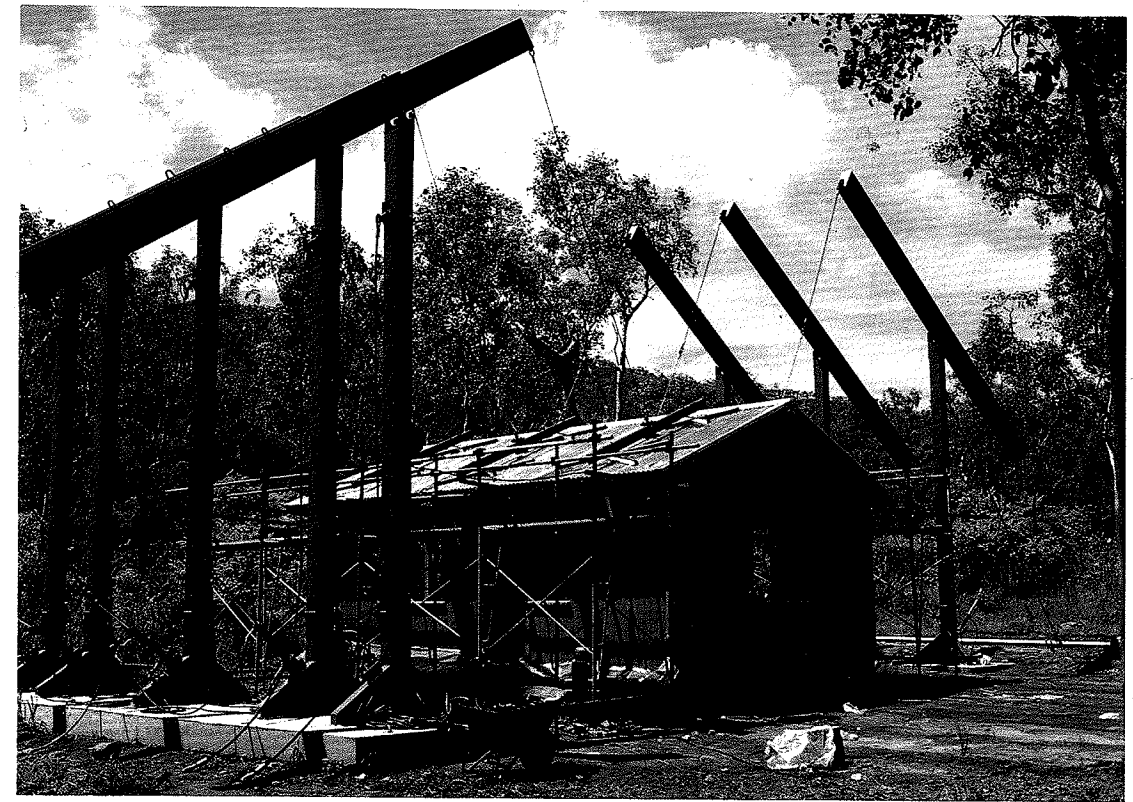
Figure 16 Cyclic loading tests on basic Tongan house
