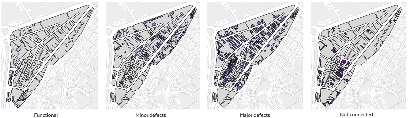
Figure 47 Condition of buildings' connection to wastewater network
