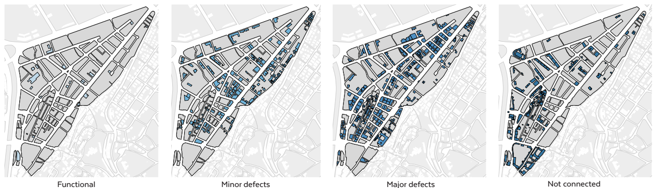
Figure 44 Condition of buildings' connection to domestic water network
