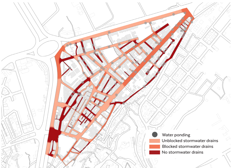
Figure 48 Street mapping of stormwater network
