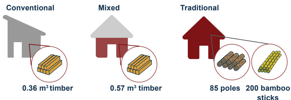
Figure 5. Quantity of material required by construction typology for one house.
