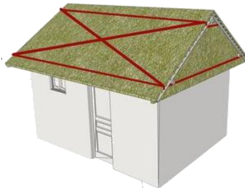
ROOF BRACING AND CONNECTIONS OF THE COVER (CGI, THATCH) TO THE ROOF STRUCTURE
