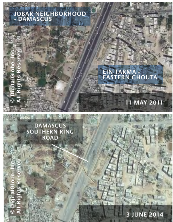
FIGURE 22 Heavy damage to the Damascus Southern Ring Road that impedes vehicle traffic in the area.
