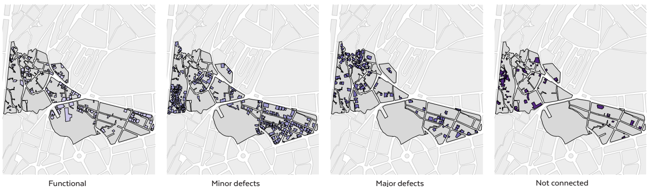
Figure 44 Condition of buildings' connection to wastewater network
