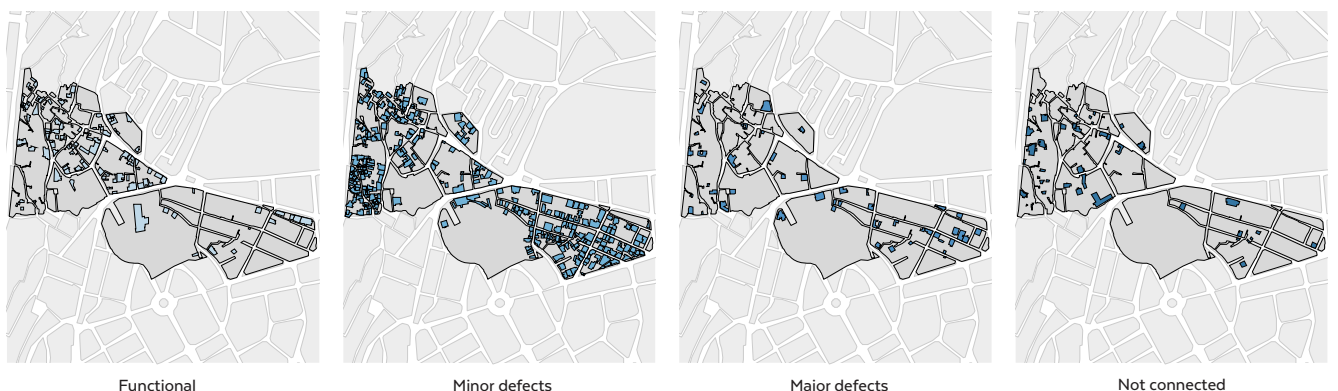
Figure 42 Condition of buildings' connection to domestic water network
