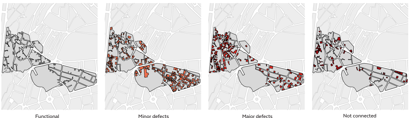
Figure 46 Condition of buildings' connection to stormwater network
