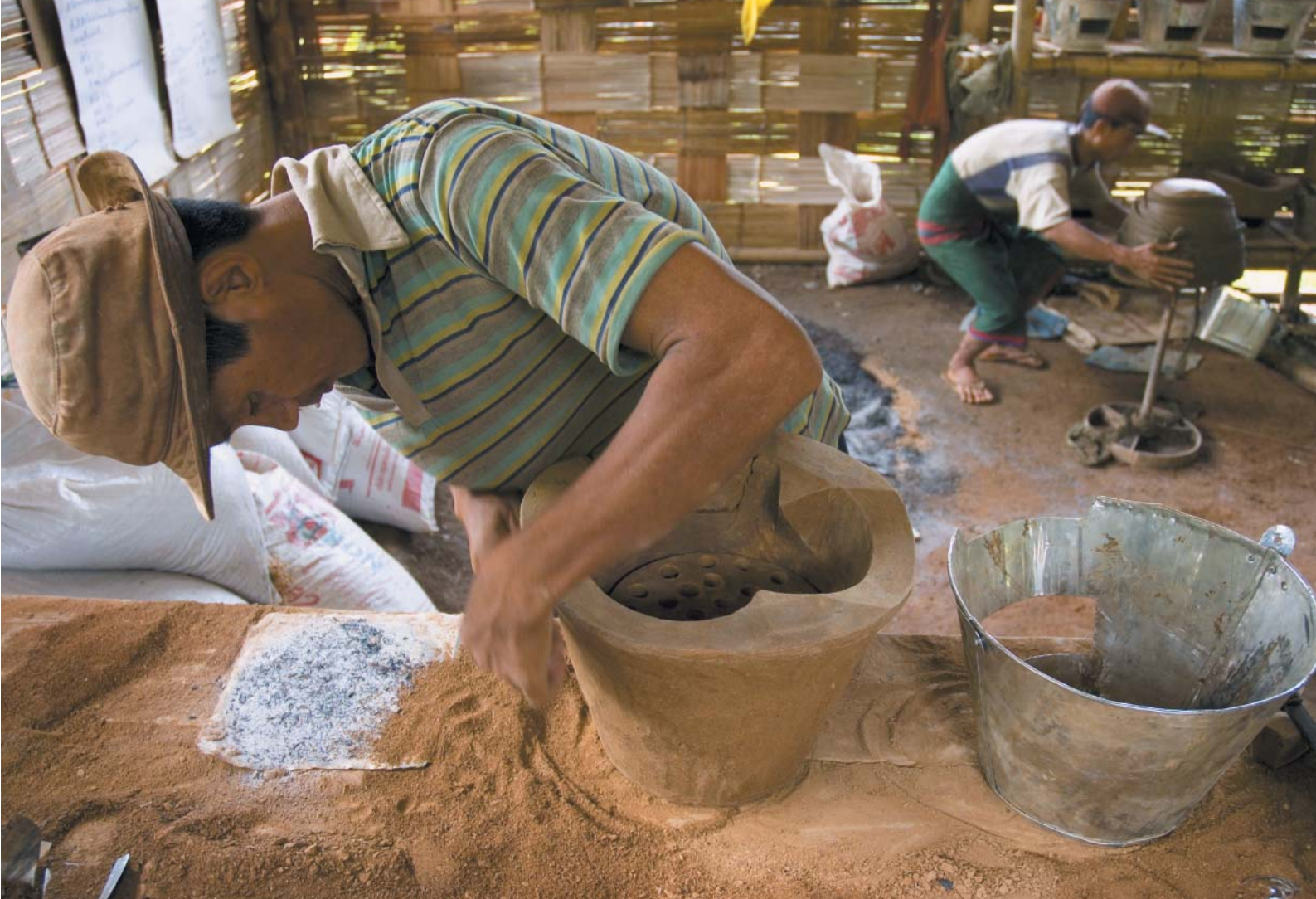
UNHCR has set up technical schools in camps to help some of the 140,000 refugees from Myanmar. Refugees learn practical skills such as clay charcoal stove making. UNHCR / J. Redfern
