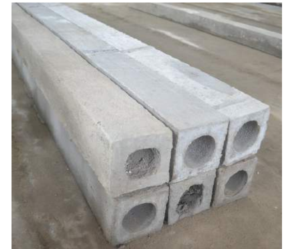
Ferrocement Hollow Column
