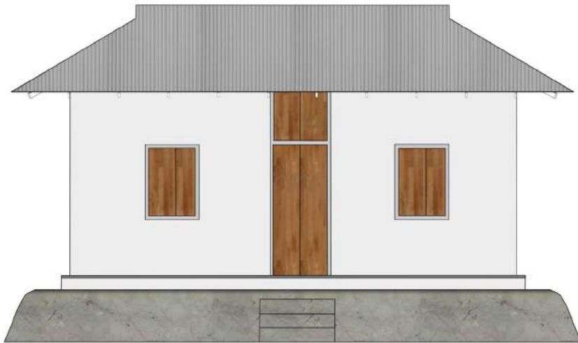
Front Elevation with Escape Door For Area 2 & 3
