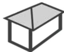
Multiple roof slopes reduce the risk of your roof being pulled apart
