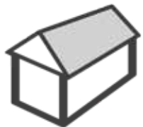
Two-sided gable roof
