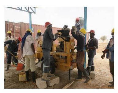
Hydraform machine in action – Brick production with a mix of clay and cement – EU Trust Fund supported project, UNHCR Diffa
