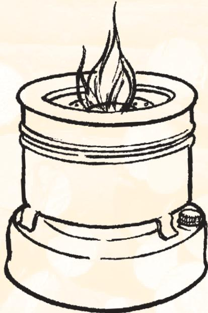
Kerosene stoves use either cloth wicks or a pressurised pump system.
