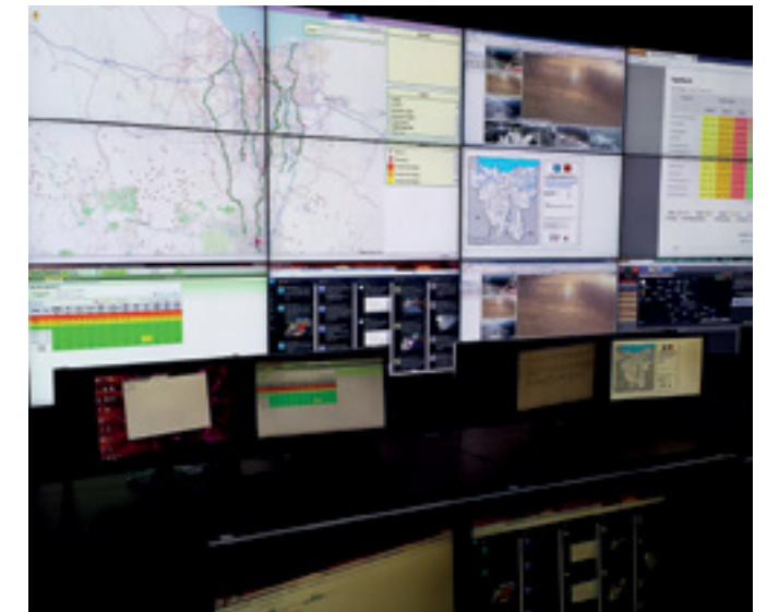
Pusdalops control center decision-making tools, including maps, real-time flood data, and live streaming camera pointed on the dam
