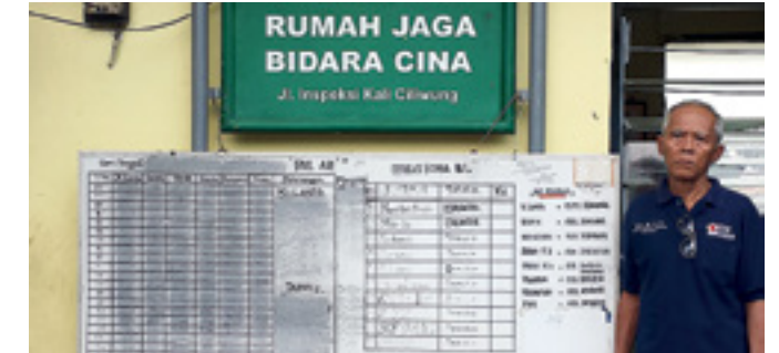
The RW (local leader) of Bidara Cina community stands next to the whiteboard where flood data is gathered and posted on the river watch house. To inform their own preparations and actions, watch house volunteers update the monitoring board every three to five minutes by calling the dam when there is a threat of a flood.
