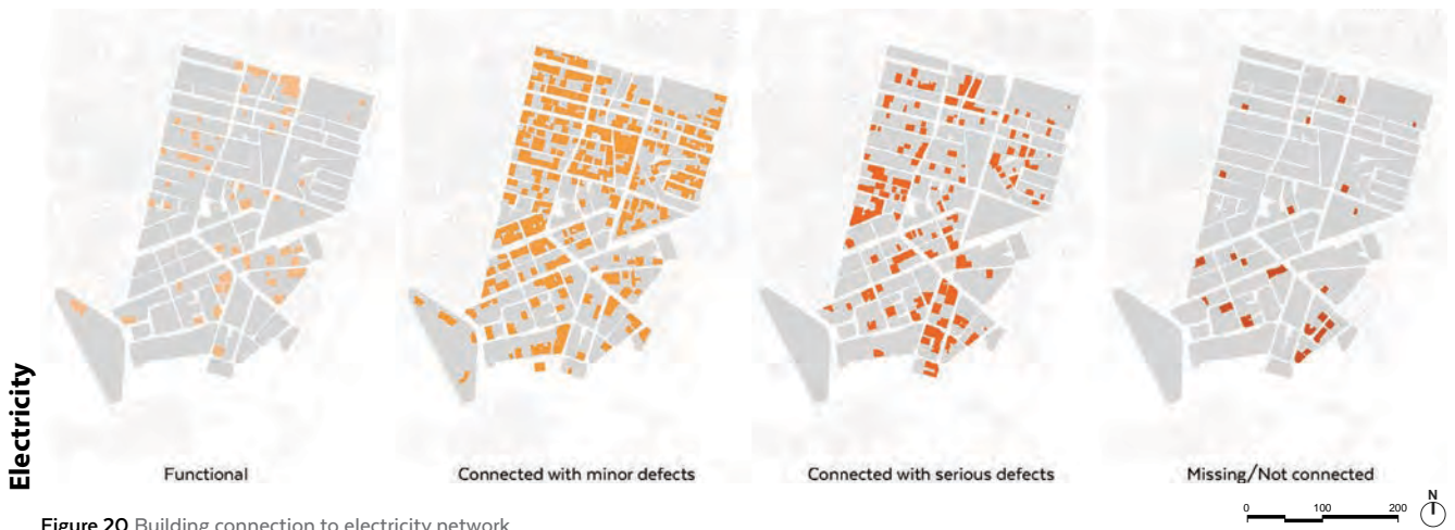
Figure 20 Building connection to electricity network
