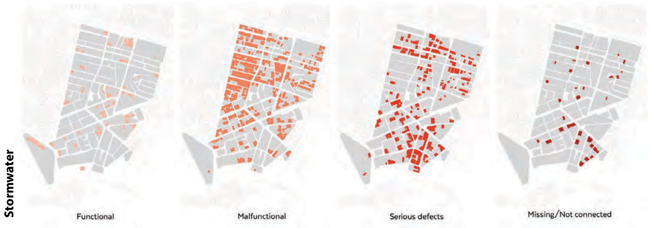
Figure 19 Building connection to stormwater network
