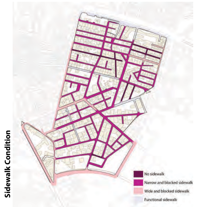
Figure 24 Sidewalk condition mapping *Sidewalks are blocked by people for private parking or by shops outspreading their merchandise.
