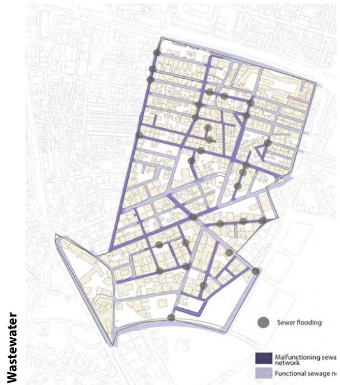
Figure 18 Wastewater street mapping
