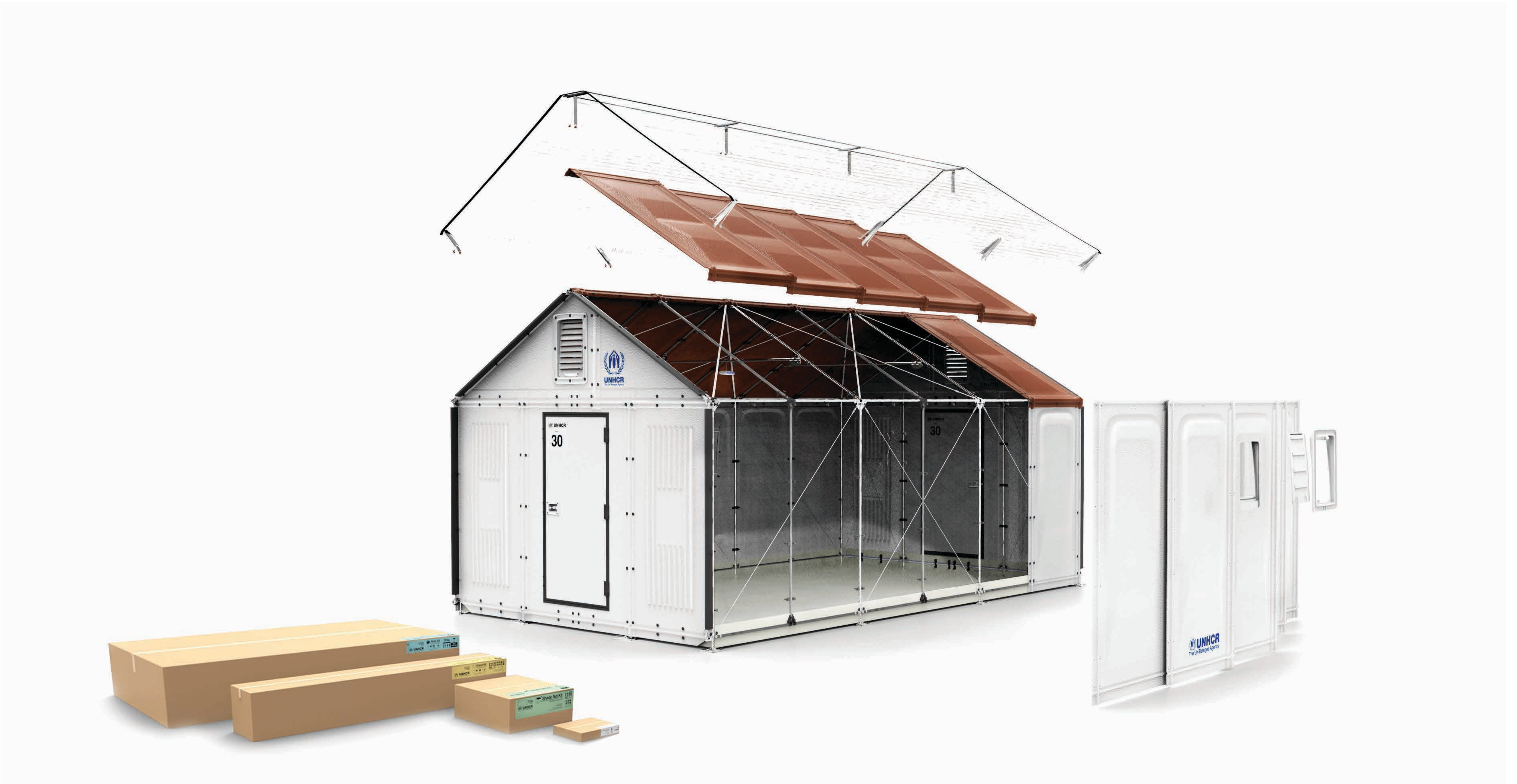
The above illustration shows the RHU Frame, RHU Panels, RHU PV System and RHU Shade Net, and their respective packages
