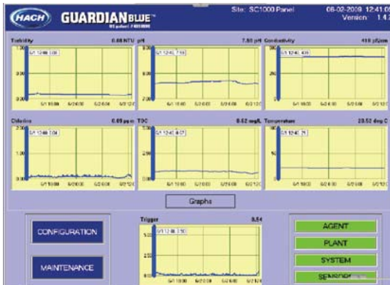
Figure 1. Online monitoring data of drinking water
