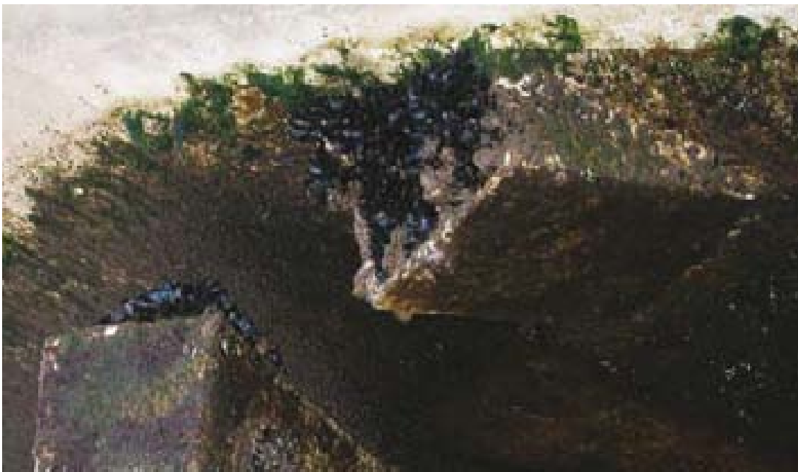
Figure 35: Antifouling paint is useful only for boats which are always in the water.
