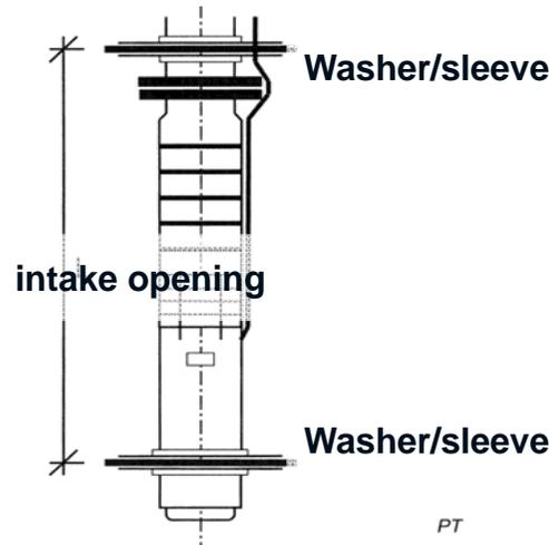
Washer/sleeve Overpumping well with a higher pumping rate than the production rate
