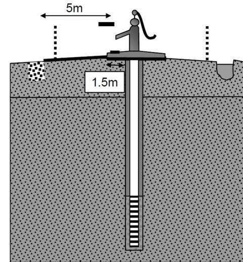
potentially contaminated surface water must not flow towards the well but must be drained away
