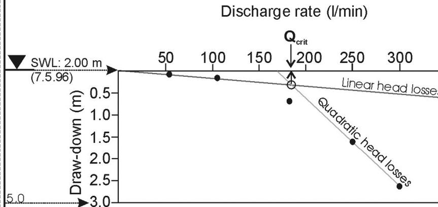
Step draw-down data measured just after construction of the 'CHYN well', Buix
