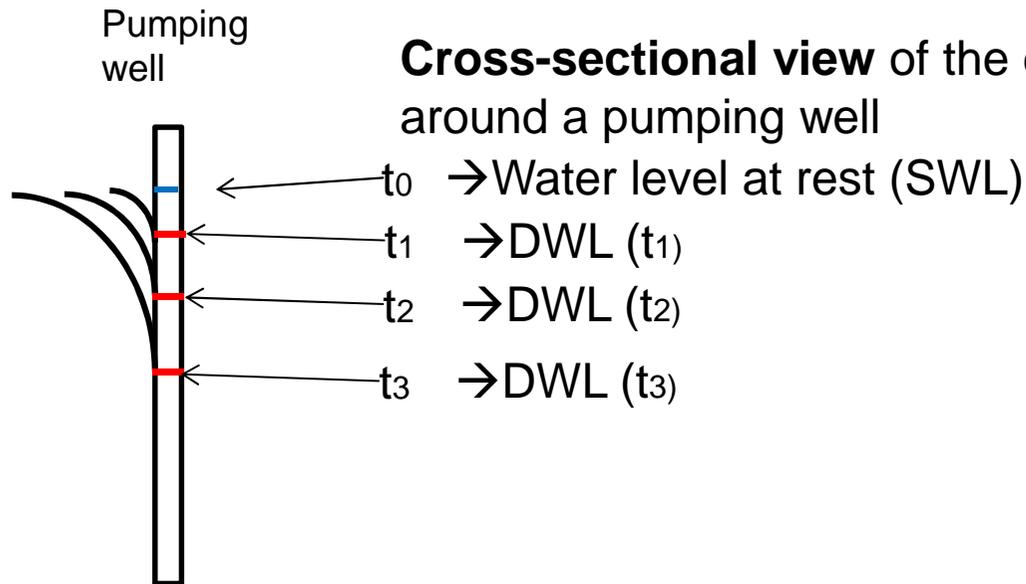
**Cross-sectional view** of the expanding depression cone with time around a pumping well
