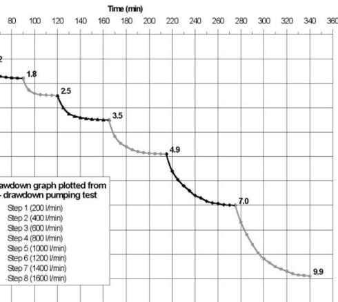
Quadratic head losses: draw-down is no longer linear to draw-down, indicating turbulent flow → encrustation of screens, inflow of particles etc.
