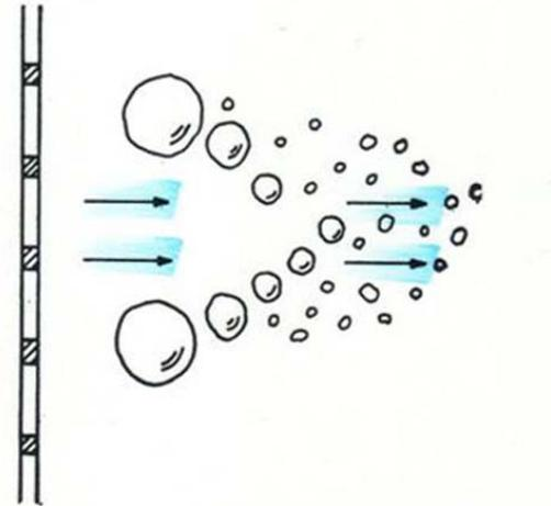
Fig. 103 Dispersal of grain arches through alternating impact desanding.
