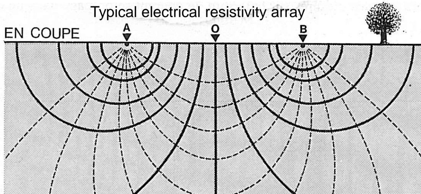
Two current electrodes A and B with the current lines (dashed) being perpendicular to the voltage equipotentials (bold lines), measured between to potential electrodes close to O.
