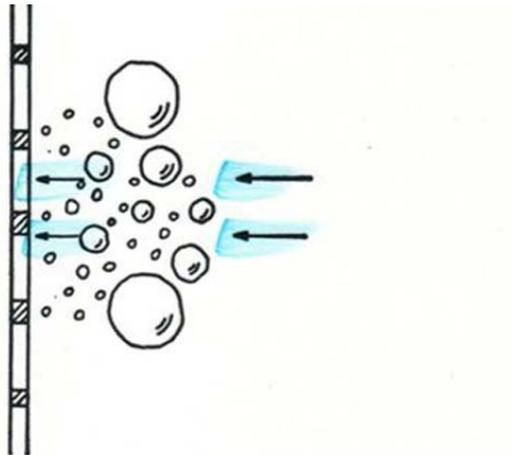
Fig. 104 The finer grains are drawn into the screen by repeated suction, following impacts.
