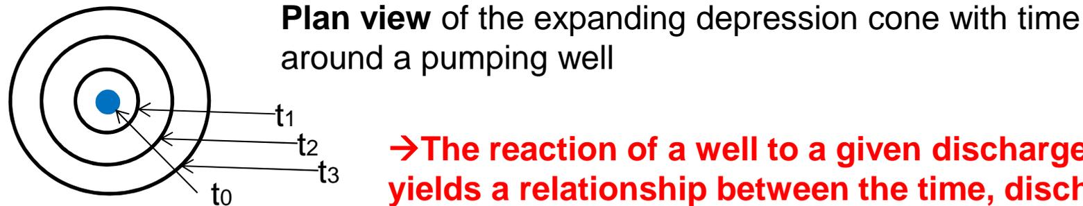
**Plan view** of the expanding depression cone with time around a pumping well
