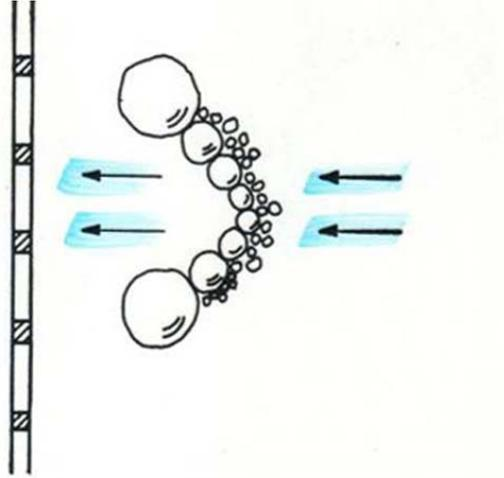
Fig. 102 Formation of grain arches caused by suction desanding in one direction only.
