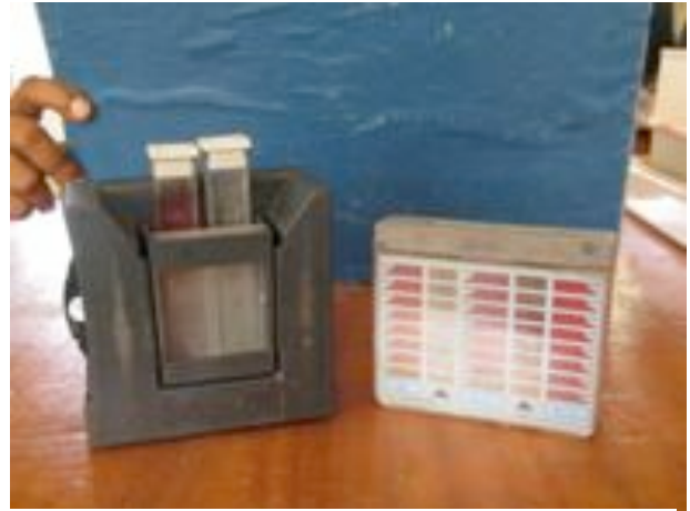
Chlorine test kits (with minor errors)
